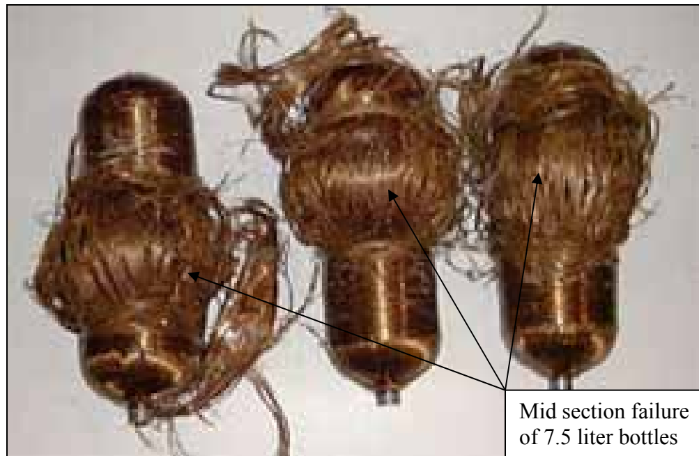
Figure 2.4 burst COPVs tested by Hypercomp Engineering Inc.
